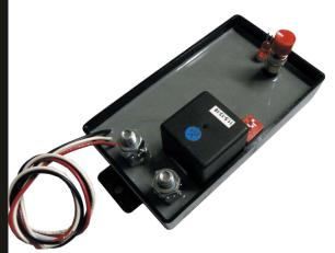
This unit is designed to protect the car battery from excessive discharge, when the ignition is off.
