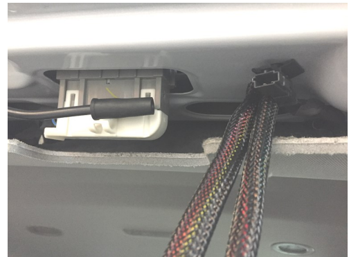
Reconnect water pipe and light connector back to its position.
